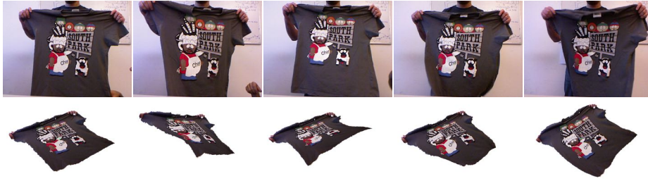
Fig. 3. Color input data of the deformation tracking method (top row) along with the deformed referenced model from a rotated point of view (bottom row).
