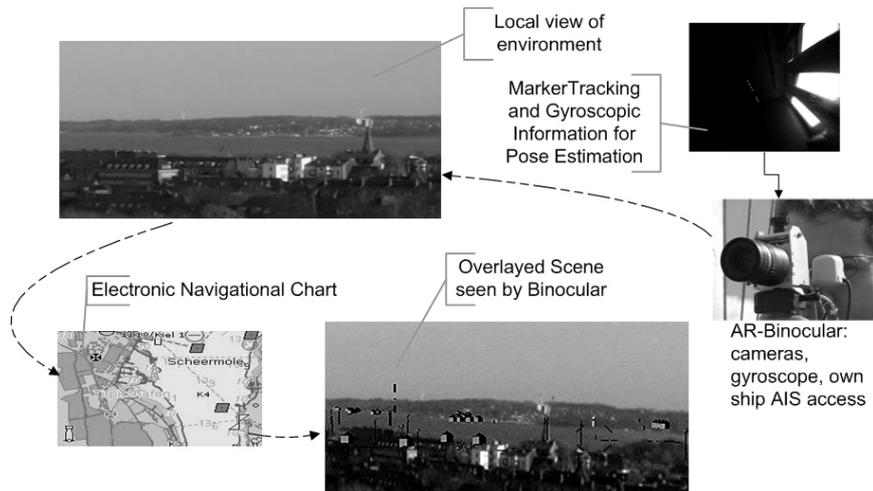
**Figure 1.** Augmentation Principle of the Augmented Reality Binocular; on the right there is a video capture and pose estimation device; it overlays the local environment (top left), with the correctly aligned chart data (bottom left).
