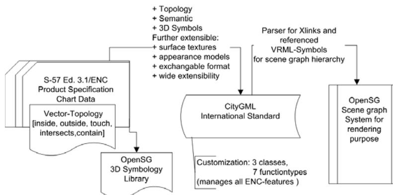
**Figure 2.** Data flow of the conversion from S-57 ENC data to CityGML and into a scene graph system.
