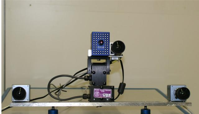
**Fig. 1.** The setup comprising of a moving PMD 2D3D-camera mounted on a pan-tilt unit between two fixed high resolution optical cameras.
