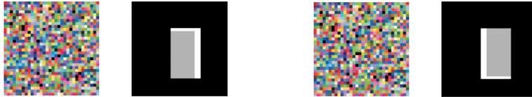
**Fig. 3.** Artificial flow sequence images (noisy images) generated by moving a 8x16 pixel block (foreground object) by 2 pixels right and one up in front of a 32x32 pixel image (containing uniformly distributed noise, pixelwise independent). Ground truth optical flow is displayed right of each image, i.e. black pixels have the same position in both images, grey ones are displaced. Pure white pixels are occluded in the other image.
