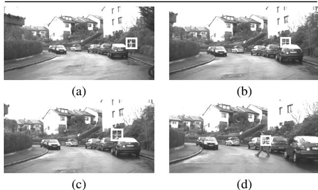
**Figure 7.** Some images from a pedestrian crossing sequence. The pedestrian is detected early and tracked, even though it is temporarily partially occluded by a parked car. A warning is issued in image (c).
