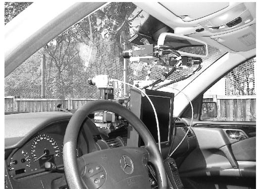
**Figure 1.** The UTA demonstrator from the Daimler Chrysler AG. Only one of the two PTU mounted cameras is used in this work.
